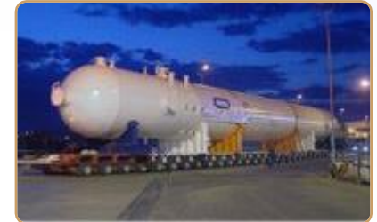
Slug Catcher Surge Vessel, Hasdrubal Project, Tunisia, PETROFAC
