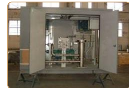
Water Injection Module, GE
