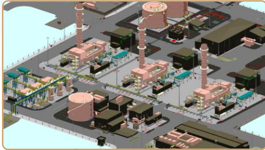
3x42 MW SCGT Power Plant, West Qurna-2 Oilfield, Iraq, ENKA
