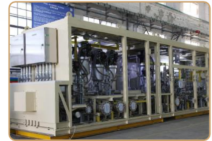
Fuel Gas Module, MHPS
